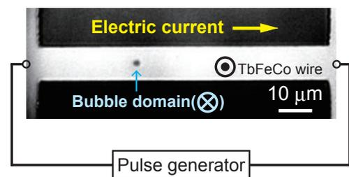
Fig. 1. A magneto-optical Kerr micrograph of a BD in a TbFeCo wire and an illustration of the experimental setup.
