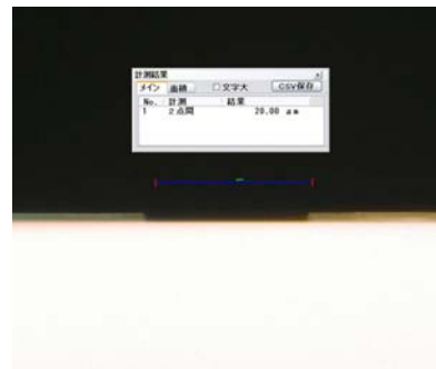
Fig.6 Optical microscopic image of photoresist (AZ1500 3.8cp) from side view
